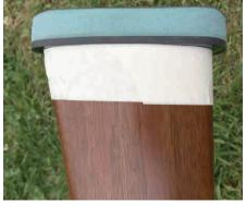
Masking tape applied before fitting.
